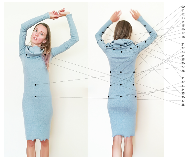
Figure 13: The vibration motor positioning on the final prototype - a tubular haptic dress. Video of the final piece: https://tinivurl.com/magiclining
