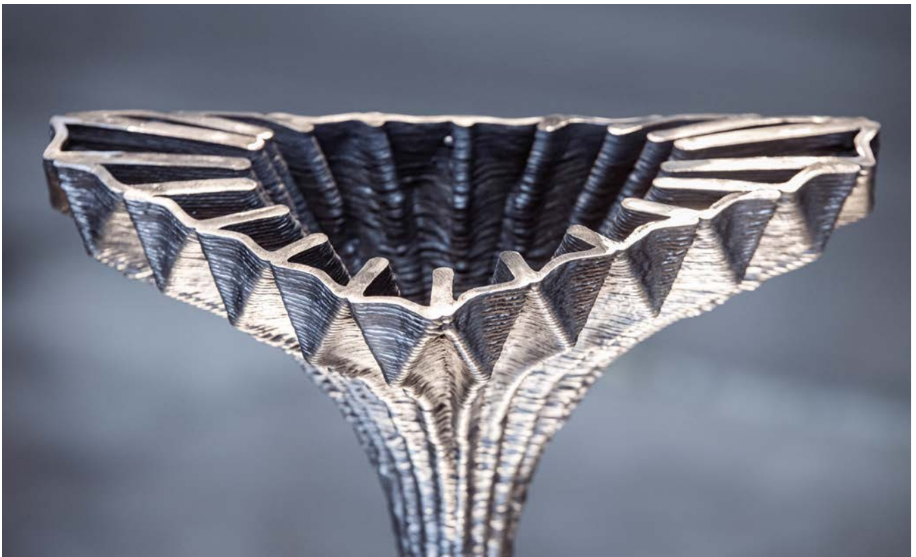
OS:WAAM (Wire Arc Additive Manufacturing) – Sebastien Wierinck
